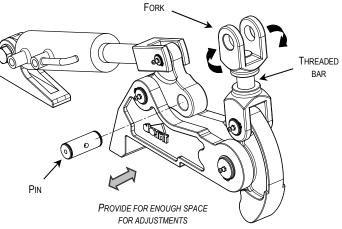
To easily adjust the clamps, during installation, it is important to leave enough space to remove the pin and one of the forks.
