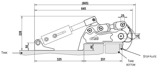
Note: the dimension between brackets refers to clamp in open condition.
