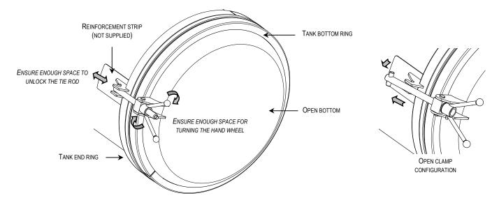
To allow for easy manual activation of the clamps, during installation, it is important to leave enough space to turn the hand wheel and unlock/remove the tie rod
