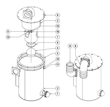
DL cyclone secondary shutoff (mild steel) - code 14450 026 E0
